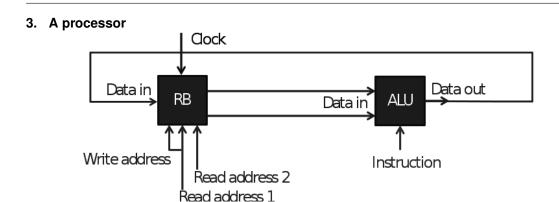
The ALU of the processor above has two instructions: 0 = add and 1 = multiply. Furthermore it has four 1-bit registers, called R0 through R3. The starting value for register R3 equals 0. Give for this processor the program for the following computation:  $R3 = R1 \times (R1 + R2)$
