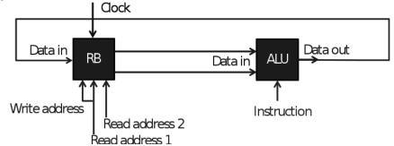
The ALU of the processor above has two instructions: 0 = `ADD' and 1 = `MUL'. Furthermore it has 4 8-bit registers. The starting value for register R4 equals 0. Give for this processor the program for computing R1 + (R2 \* R3) + R1 and storing the result into R1. (You may not need all timeslots.)
