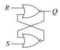
Is this synchronous sequential logic?
